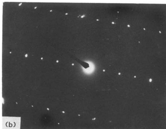
Figure 7 (a) Dark-field electron micrograph of a cementite islet obtained with the (001)_{Fe_3C} diffracted beam; (b) electron diffraction pattern of the same area. [1\bar{1}3]_\alpha and [2\bar{1}0]_{Fe_3C} Laue-zones.
